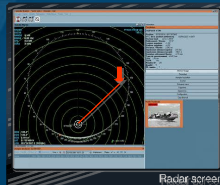
3 Simultaneous display of position and image on map or radar screen and viewer
